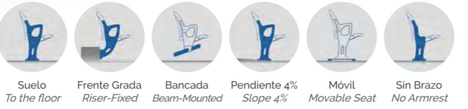
Suelo To the floor      Frente Grada Riser-Fixed      Bancada Beam-Mounted      Pendiente 4% Slope 4%      Móvil Movable Seat      Sin Brazo No Armrest
